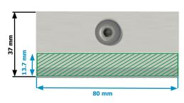
**Maximum clamping surface LEC:** A=13.7\*80=1096mm<sup>2</sup> (top and bottom)
