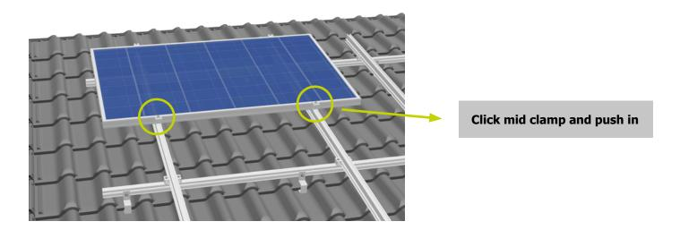
Now slide the next module underneath the mid clamp, adjust the mid clamp to the height of the module's frame and tighten the screw (tightening torque 8-10 Nm).
