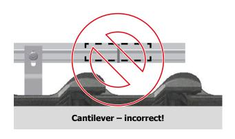
Position the splices between two roof hooks.
