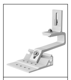
The bracket is rotated by 90° for the horizontal rail connection. Loosen nut, rotate bracket and ribbed plate by 90° and re-tighten nut (tightening torque 12–15 Nm)
