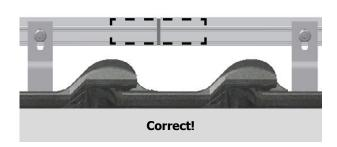
If the mounting rail is longer than 13.20 m, the module array must be separated by placing two end clamps.
