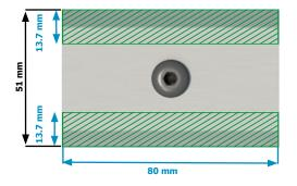
**Maximum clamping surface LMC:** A=13.7\*80=1096mm<sup>2</sup> (per side, top and bottom)
