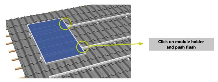
Align the upper row of modules with the aid of a guide or levelling instrument.
