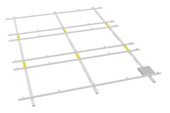
All ground rails have covering cable duct receptacles to protect the string lines from permanent and harmful environmental influences, in particular UV radiation. Installation of the covering cable ducts is possible after every work step of the system installation. The covering cable duct is installed after the cable routing.
