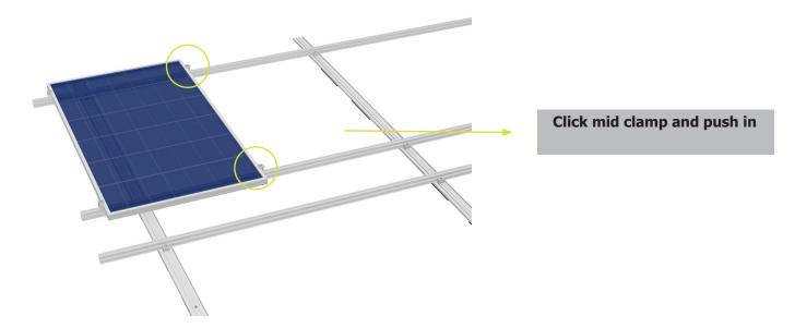
Now push the next module under the mid clamp, adjust the mid clamp to the height of the module frame and tighten the screw (torque 8-10 Nm).
