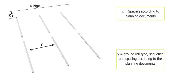
All ground rails are provided with an 11 mm thick high-tech protective foam mat. This ensures a free water drainage and prevents damage to the roof covering due to mechanical impacts and long-term damage from plasticiser migration.
