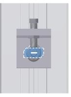
bracket hammerhead bolt M8x25 self-locking Attach the mounting rail to the using а and а bolts are correctly aligned in the mounting rail channel nut. Ensure that the hammerhead
