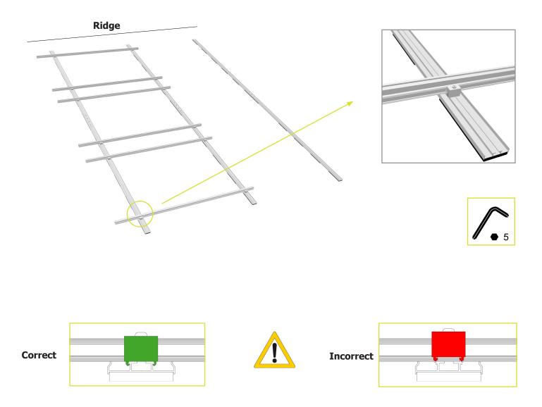
2.3.2 Rail ST-AK 7/47 using bracket 40 mm M8 (for sandwich roofs)
