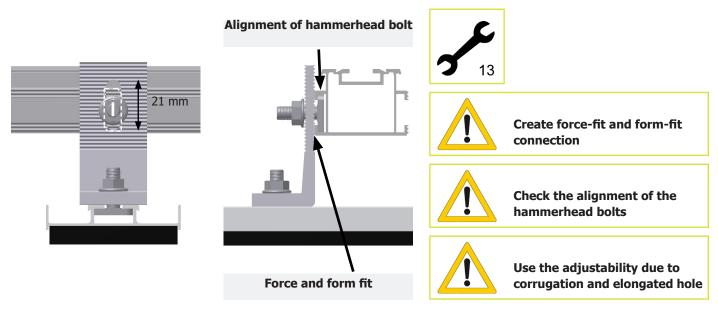
It is important to ensure that the groove in the hammerhead bolt is perpendicular (at right angles to the rail) after installing the clamp. Only then is the head of the hammerhead bolt correctly inserted in the rail and the bracket is correctly attached.
