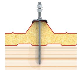
Sandwich profiles: Solar fastener Type A
