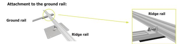
Mount the bracket 60 mm M10 onto the ground rail using a hammerhead bolt M8x25 and a self-locking nut. Ensure that the hammerhead bolt is correctly aligned in the ground rail channel (torque 12-15 Nm).
