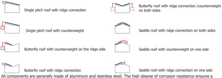
All components are generally made of aluminium and stainless steel. The high degree of corrosion resistance ensures a long service life and offers the possibility of complete recycling.
