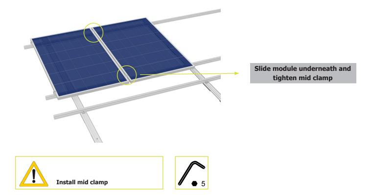
Ensure that the mid clamp clamps both of the module frames on the clamping area defined by the module manufacturer.
