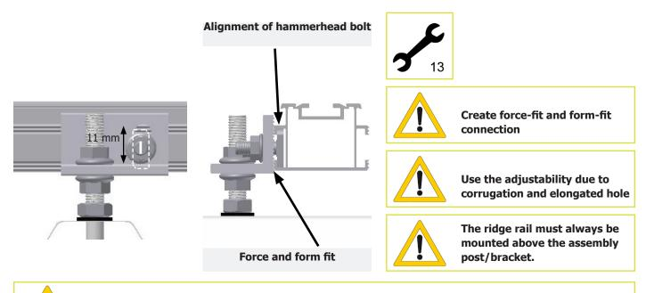
It is important to ensure that the groove in the hammerhead bolt is perpendicular (at right angles to the rail) after installing the clamp. Only then is the head of the hammerhead bolt correctly inserted in the rail and the bracket is correctly attached.
